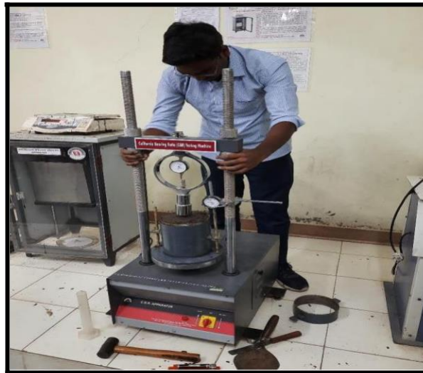
Image 3: Performing CBR on modified soil
