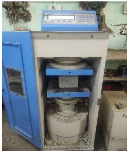
Fig-3: Block Testing Compressive strength of concrete (7 days)
