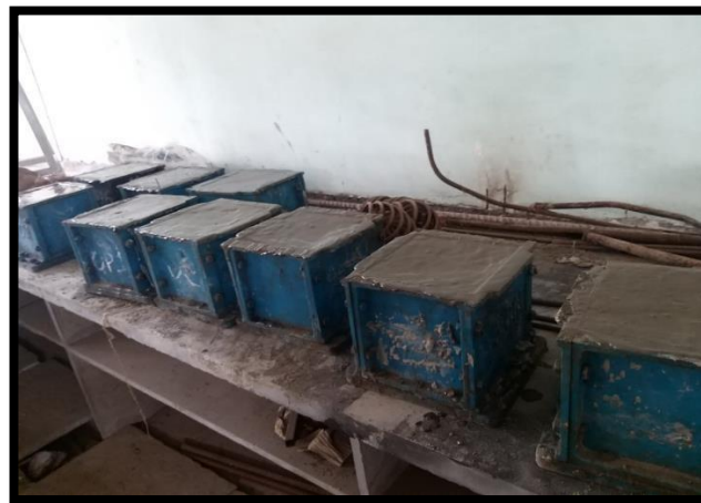
Fig -1: cube casting
