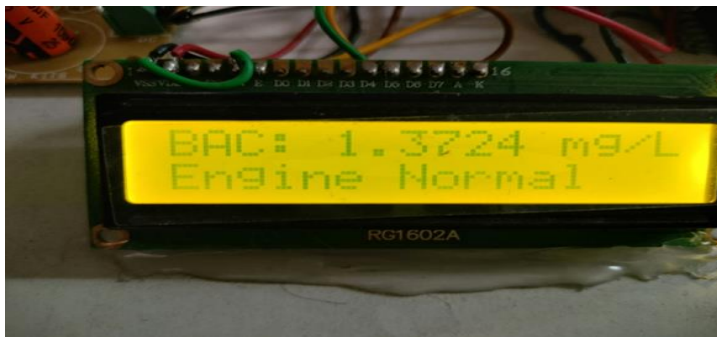
Fig: LCD when alcohol consumption is within limit
