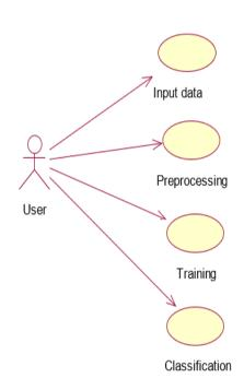
This diagram delivers graphical outline of the system functionality. System asks user for input, it will be preprocessed, and the system will be trained, and the URL features will be extracted after which the system classifies whether the given URL as input is malicious or not.
