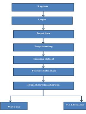
The data flow diagram (DFD) explains the flow of the system. As user enters the system it asks for the user to register and then login. After providing the input, it will be pre-processed (The following steps in pre-processing are: URL features will be extracted and then will split tokens by using vectorizer.), and the system will be trained and the URL features will be extracted after whichthe system classifies whether the given URL as input is maliciousor not.
