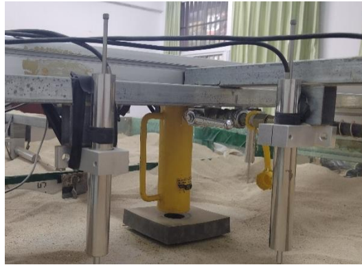
Figure 3 Composition diagram of loading and unloading system
