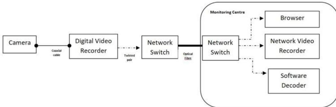
**Fig. 3: Schematic diagram for transmission of video using DVR**
