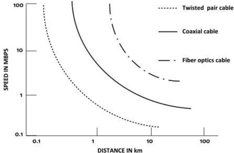
**Fig. 4: Speed vs. distance for coaxial, twisted pair & optical fibre cable**
