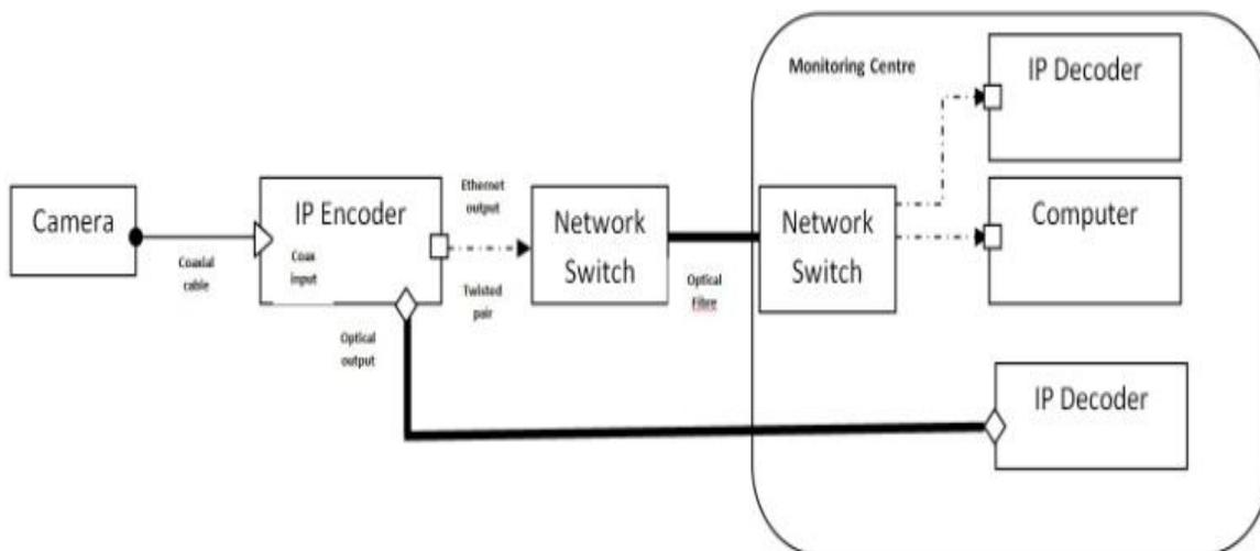
**Fig. 2: Schematic diagram for transmission of video using IP encoder**
