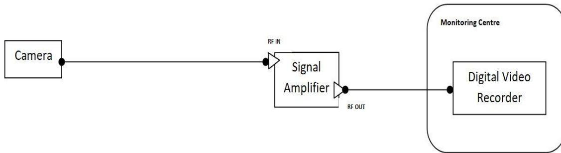
**Fig. 1: Schematic diagram for transmission of video using coaxial cable**
