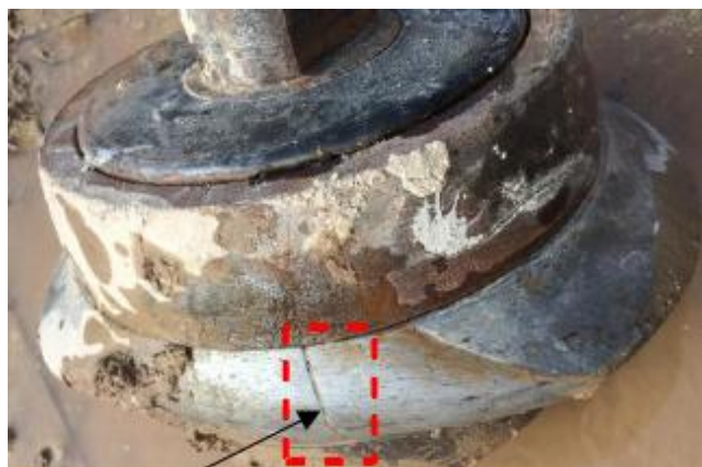
Fig.5 Phenomenon of fractured and non-uniform cutter wear
