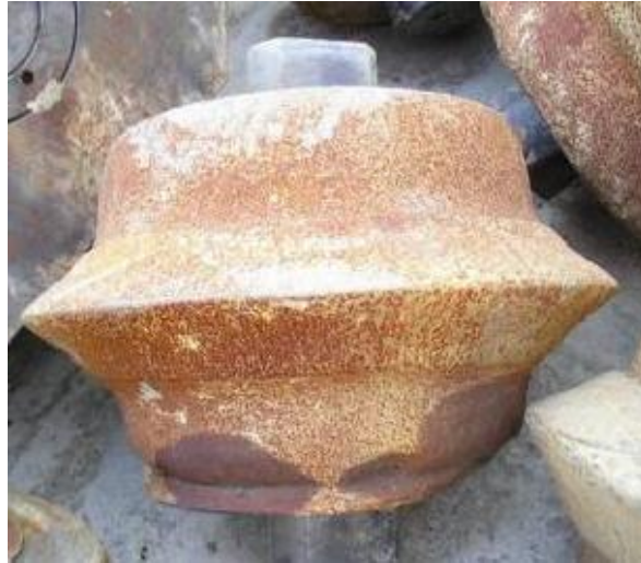
Fig.4 Phenomenon of self-sharpened cutter ring
