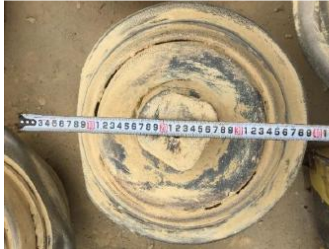
Fig.2: Phenomenon of wear occurring on local region of cutter ring
