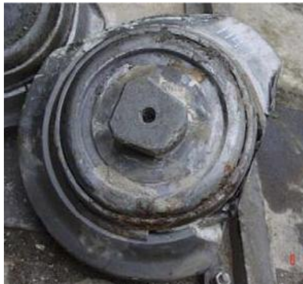
Fig.3: Phenomenon of cutter ring breakage
