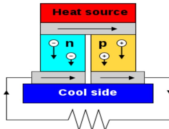
Fig: Principle diagram of TEG
