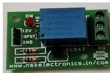
Fig:9 1-Channel Relay
