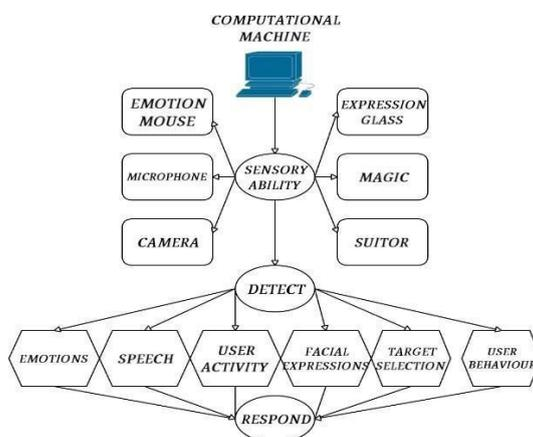
Fig1. Basic architecture of Blue Eyes Technology
