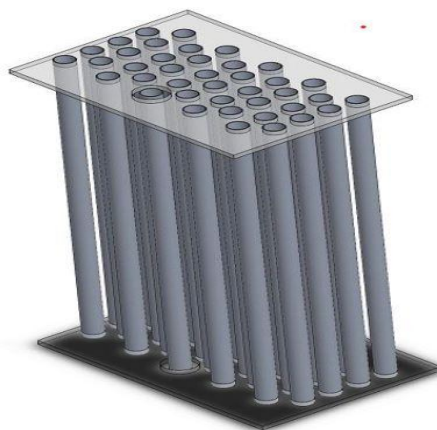
Fig 9 Tube bundle CAD Model with parallel triangular arrangement with P/D of 1.54
