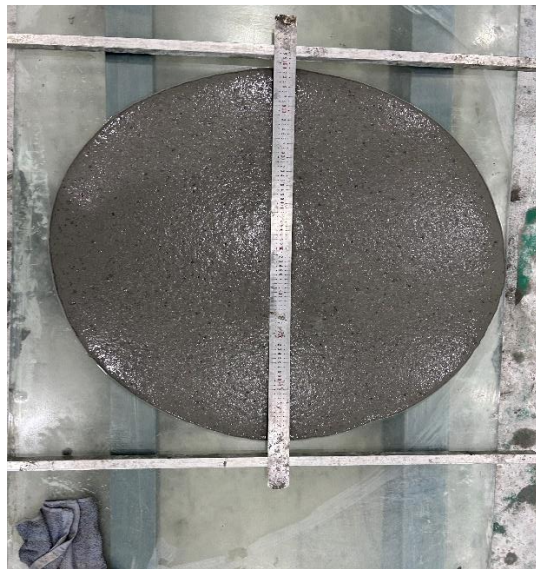
Figure 1:PCECM Fluidity Test
