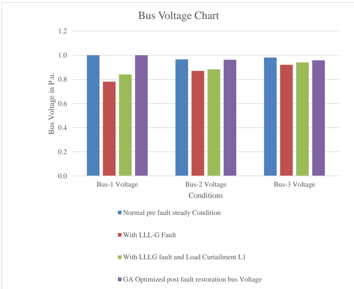
Figure 17: Bus Voltage Chart with different Scenario.
