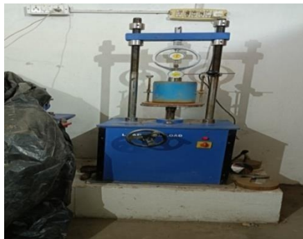
Penetration plunger of 50mm diameter
