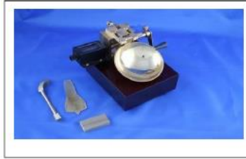
Fig.4 Casagrande Apparatus Table 4 Table for liquid limit
