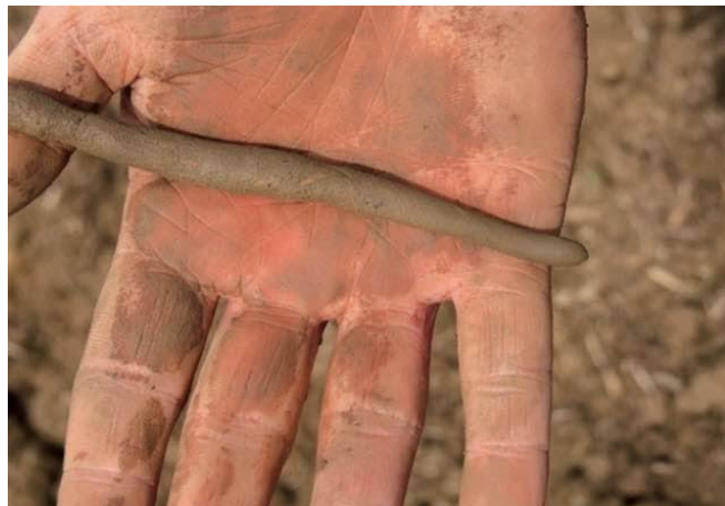
Fig.3 Plastic limit testing
