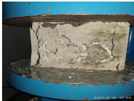
Fig. 3.6 Cracks In Cube After Compression Test
