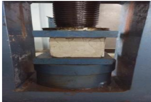
Fig. 3.5 Compression Testing On Cube Specimen
