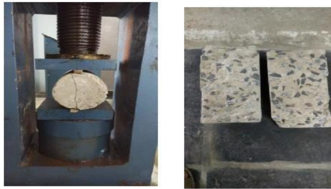
Fig. 3.8 Split Tensile Testing And Specimen (Cylinders)
