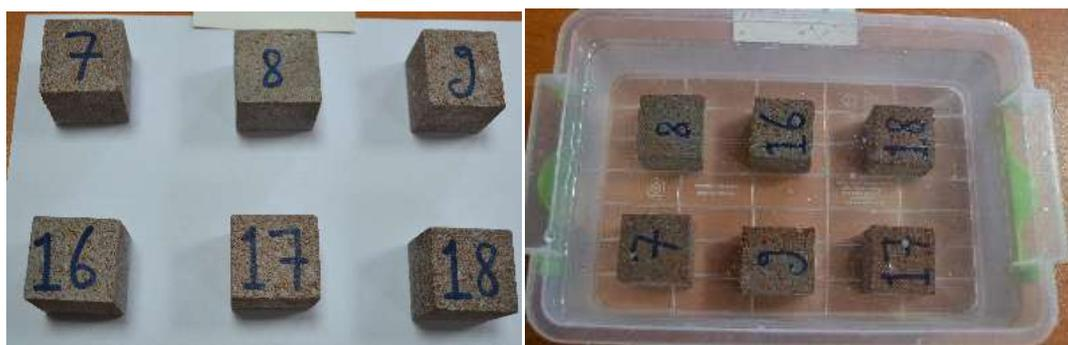
Fig. 1. Andesite samples (a. after salt contamination cycle, b. in deionized water)
