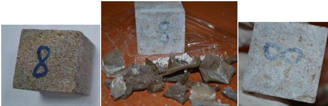
**Fig. 5.** Situation after the first clay paste cleaning cycle of sample 8 (a. Before cleaning applicationb.The sample and clay paste c. After cleaning application)
