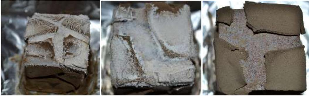
**Fig. 4.**  $\text{Na}_2\text{SO}_4$  crystals after clay-paste cycles ( a.Firstb.Secondc.Third)
