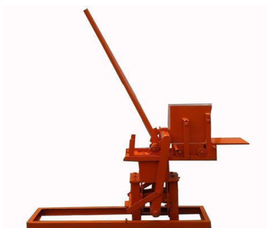
Figure 3 Manually operated brick making machine
