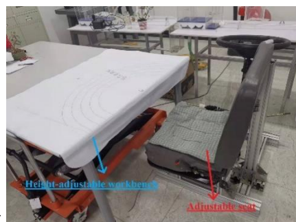
Figure 5: Arm comfort test device diagram Figure 6: Leg comfort test device diagram
