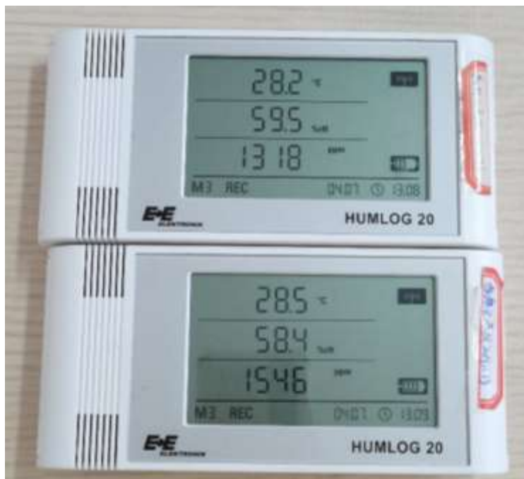
Fig. 2HUMLOG 20 carbon dioxide analyzer
