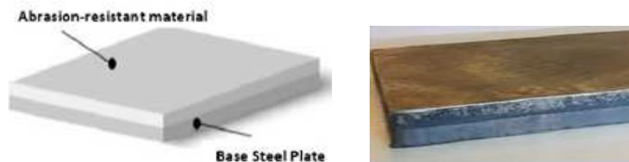
Fig 6.1&2: Picture of Cast fused steel liner (10mm base steel plate +10mm abrasion resistance material)
