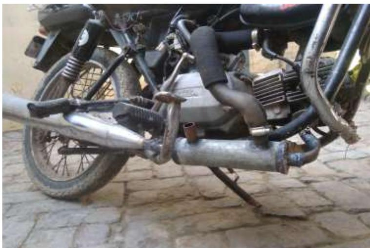
**Figure4. Air Preheater Attached with Engine Silencer**
