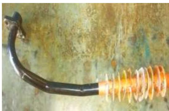
**Figure 2: Copper fins placed on copper pipe and attached with exhaust pipe.**
