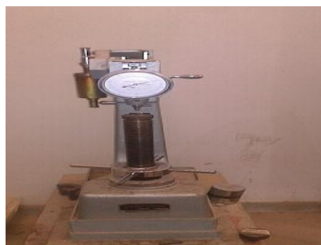
Figure 5. Rockwell Hardness Testing Machine.
