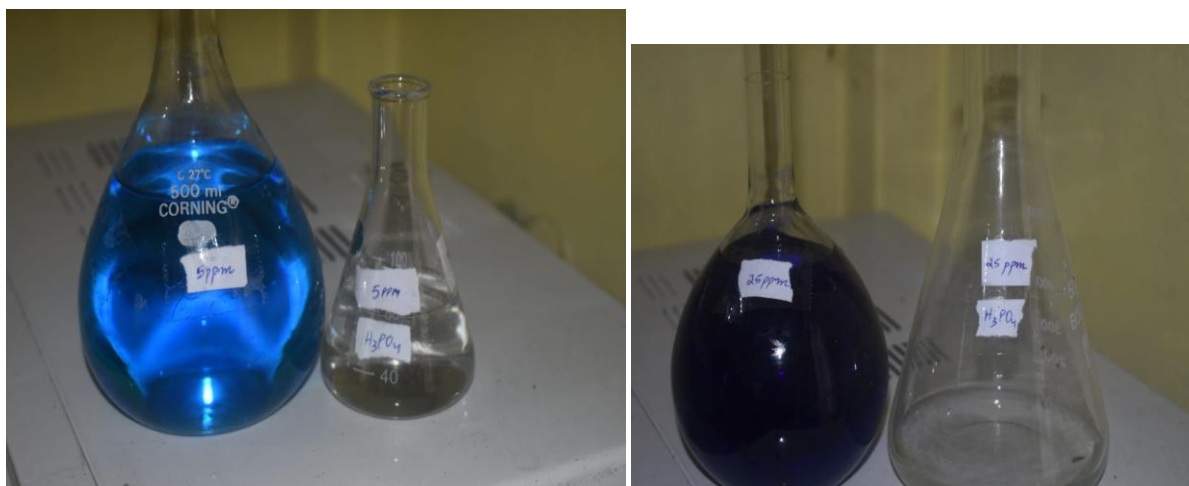
Fig 2: Images of methylene blue dye solution of different concentration: (a)5mg/L, (b)25 mg/L.(Before and after adding adsorbent).
