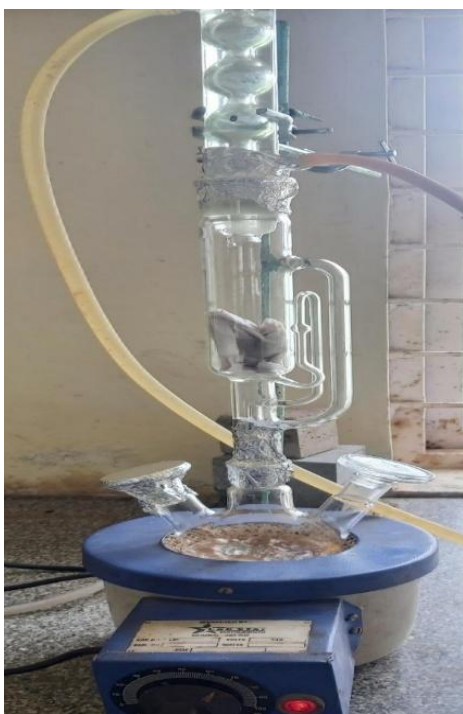
Fig. 4.20: Soxhlet process for extraction of fat
