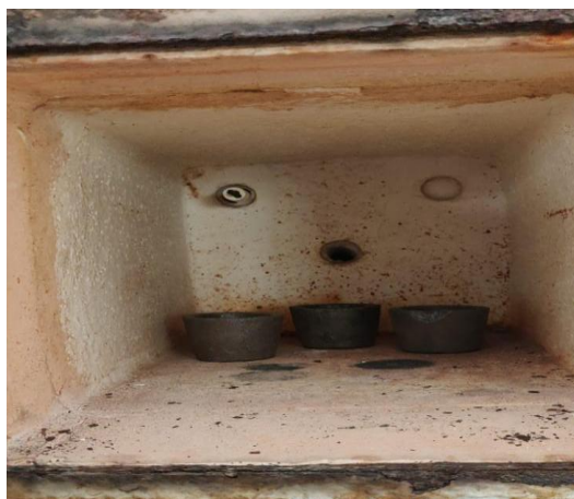
Fig 3.19 Muffle furnace apparatus
