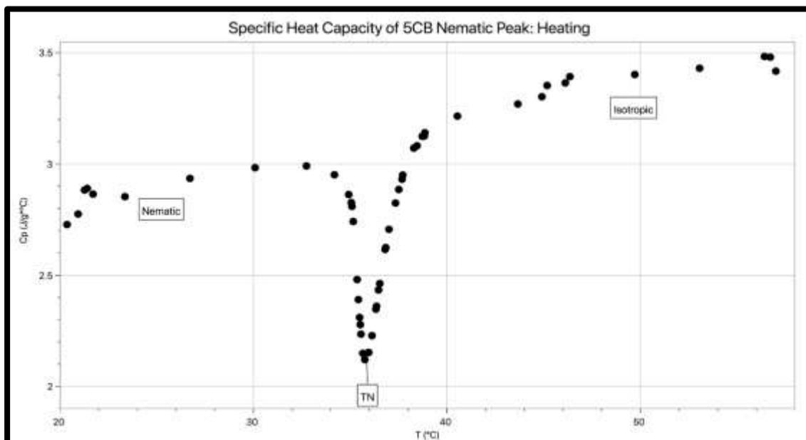
**Figure 19:** The specific heat capacity of the nematic peak from heating 5CB.
