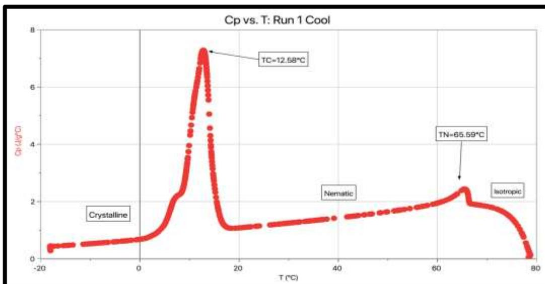
**Figure 9:** Specific heat capacity vs temperature plot for the first run's cooling only.
