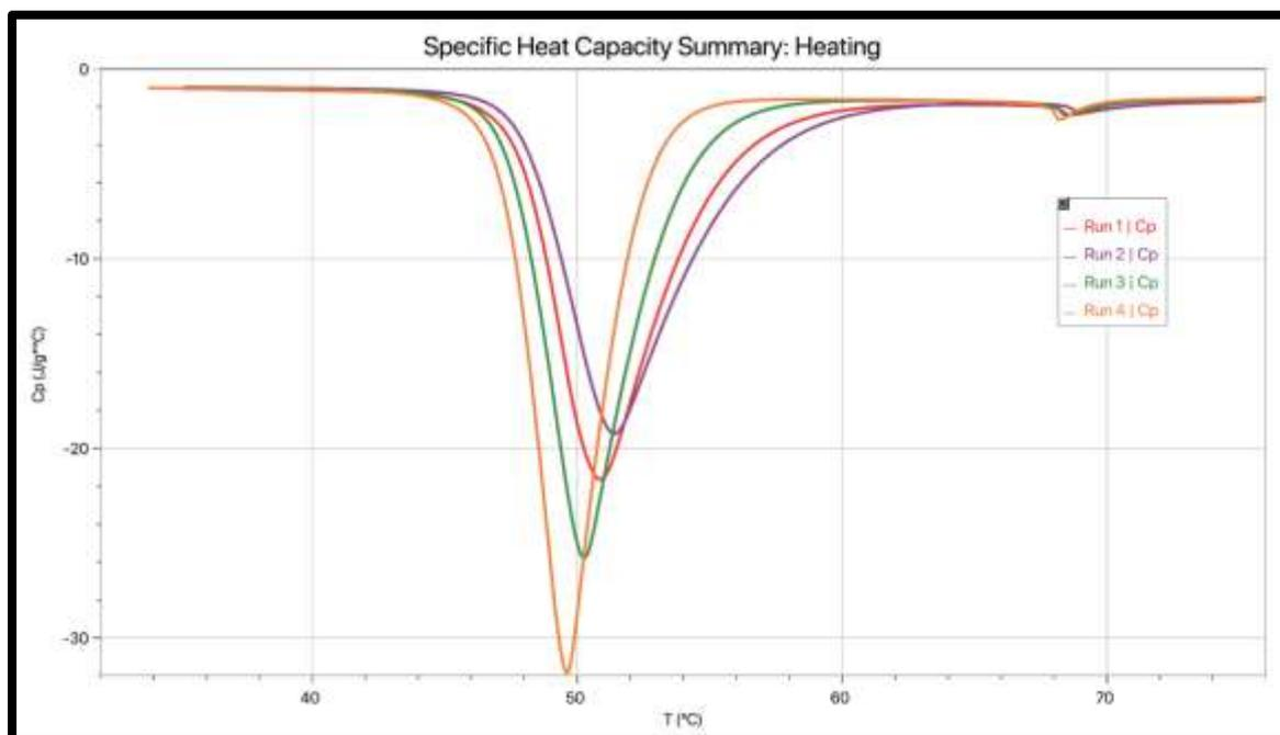
**Figure 21:** Specific heat capacity of 5OCB for all 4 runs for heating.
