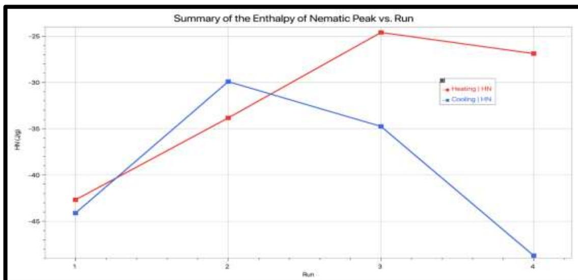
Figure 28: Enthalpy of the nematic peaks of 5OCB for the heating and cooling of all runs.
