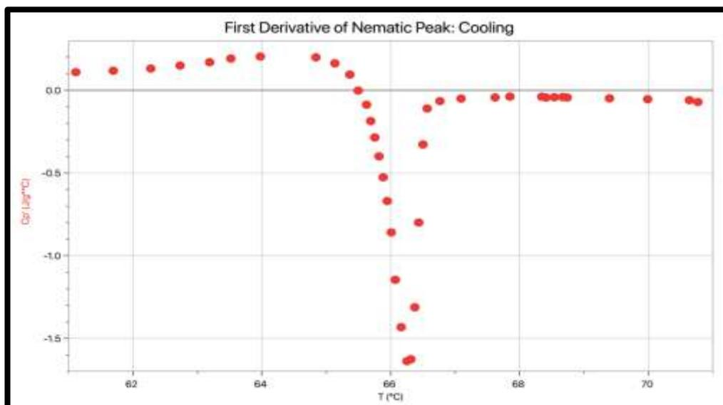
Figure 16: The first derivative of run 1's nematic peak during cooling of 5OCB.
