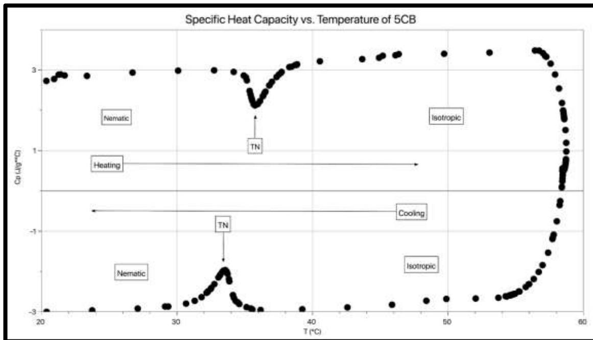
**Figure 18:** The specific heat capacity vs. temperature of 5CB being heated and cooled.
