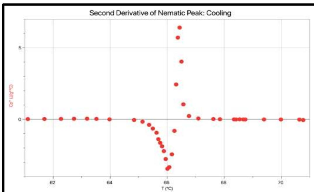
Figure 17: The second derivative of run 1's nematic peak during cooling of 5OCB.
