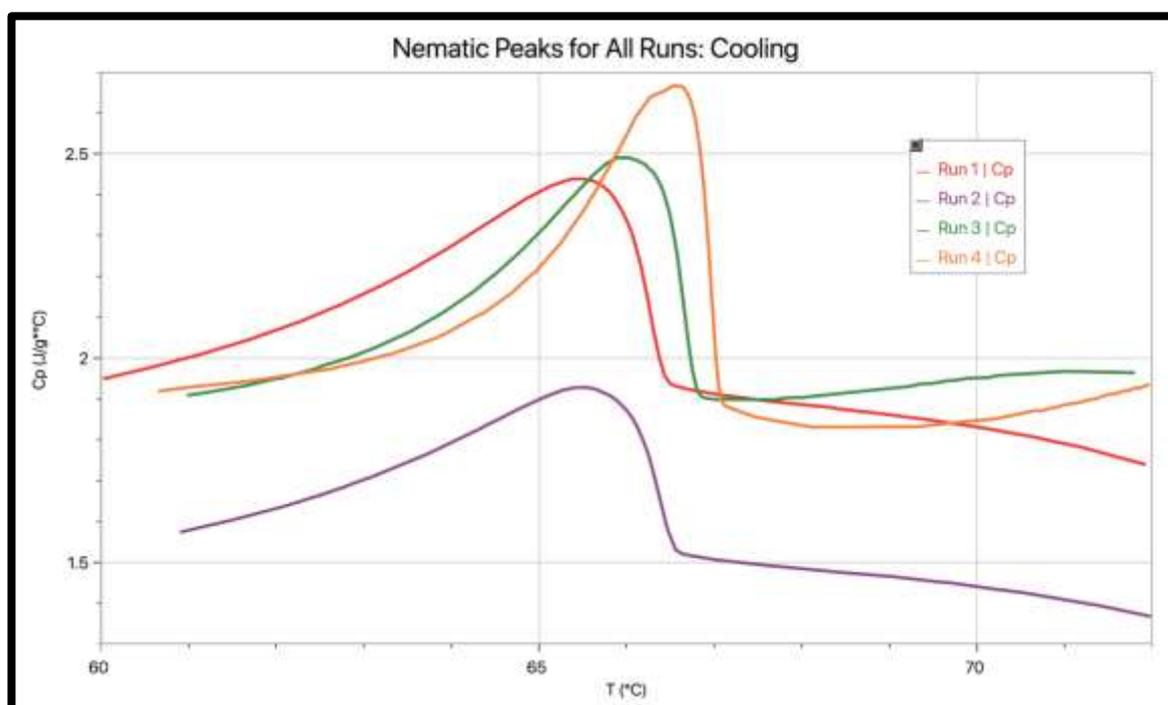
Figure 24: The zoomed in peak for the nematic peak for all runs of 5OCB being cooled.
