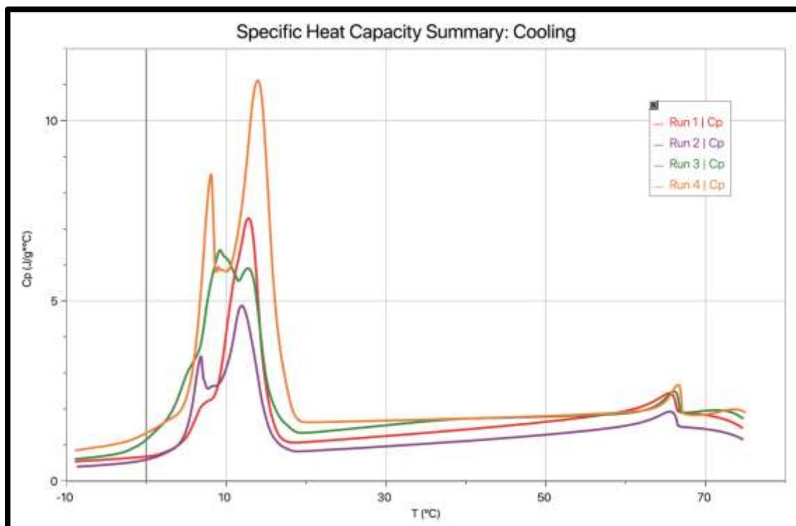
Figure 22: Specific heat capacity of 5OCB for all 4 runs for cooling.
