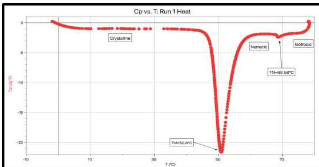
Figure 8: Specific heat capacity vs temperature plot for the first run for heating only with peak temperatures.
