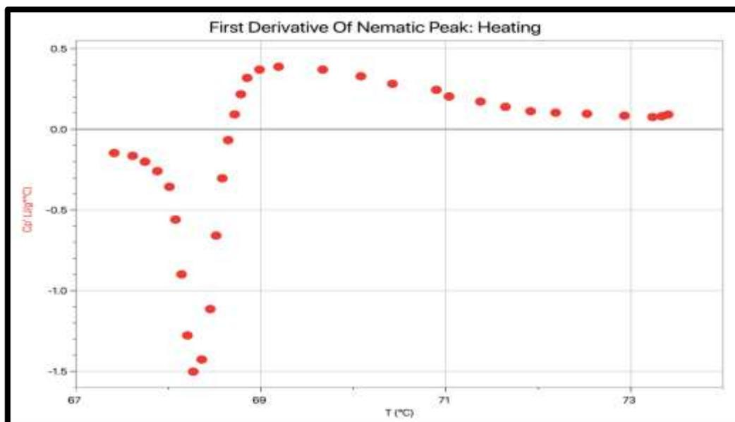
**Figure 14:** The first derivative of run 1's nematic peak during heating of 5OCB.
