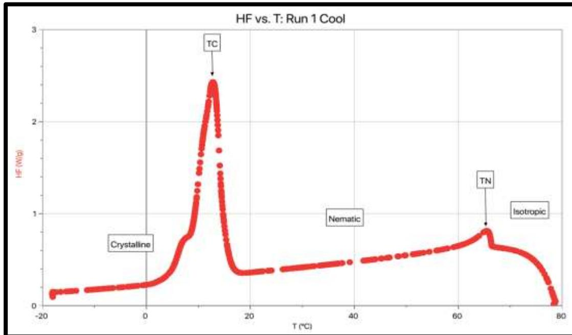
Figure 7: Normalized heat flow vs temperature plot for first run for cooling only.
