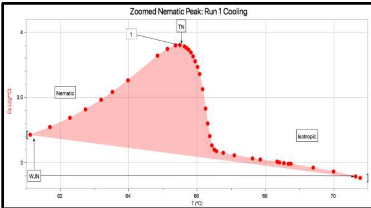
Figure 13: The enthalpy of the nematic peak for 5OCB's first run during cooling.
