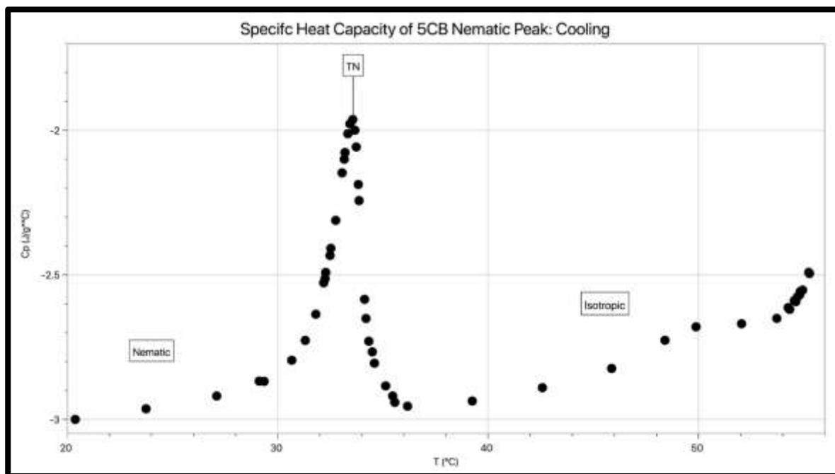
**Figure 20:** The specific heat capacity of the nematic peak for the cooling of 5CB.
