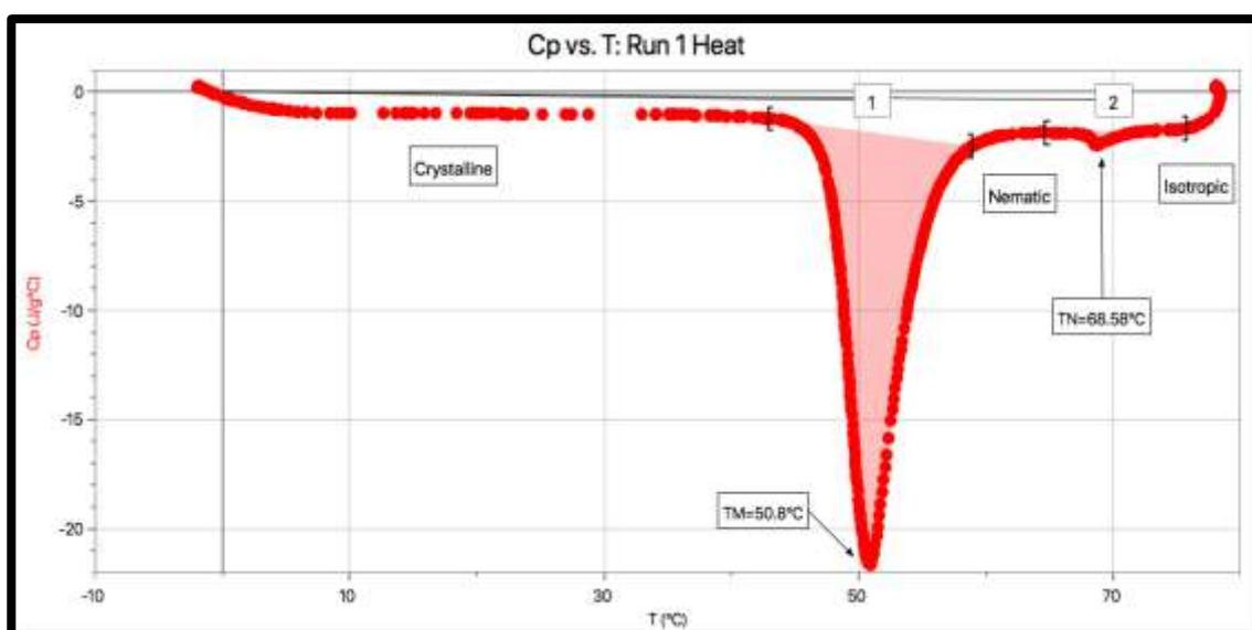
**Figure 10:** Enthalpy of the melting and the nematic transitions during heating for run 1 of 5OCB.
