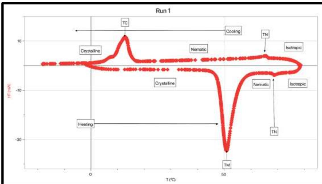
**Figure 5:** Heat and cool of 5OCB LC for the first run using the DSC plotted as heat flow Vs temperature plot.
