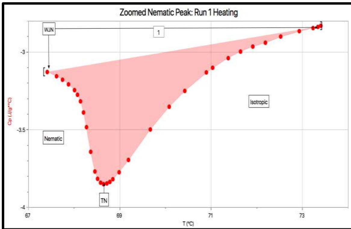
Figure 12: Enthalpy of run 1's nematic peak for heating of 5OCB.
