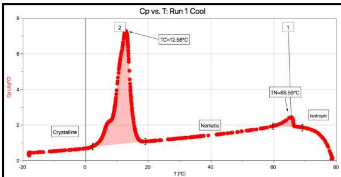
**Figure 11:** Enthalpy of nematic and crystalline peaks for run 1's cooling.
