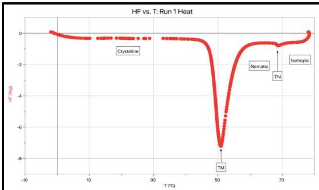
**Figure 6:** Normalized heat flow vs temperature plot for first Run for heating only.
