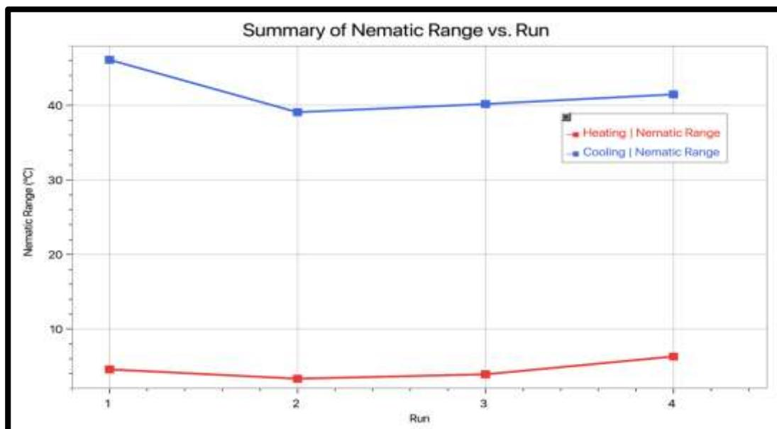
**Figure 26:** Summary graph of 5OCB’s nematic range for heating and cooling for all four runs.
