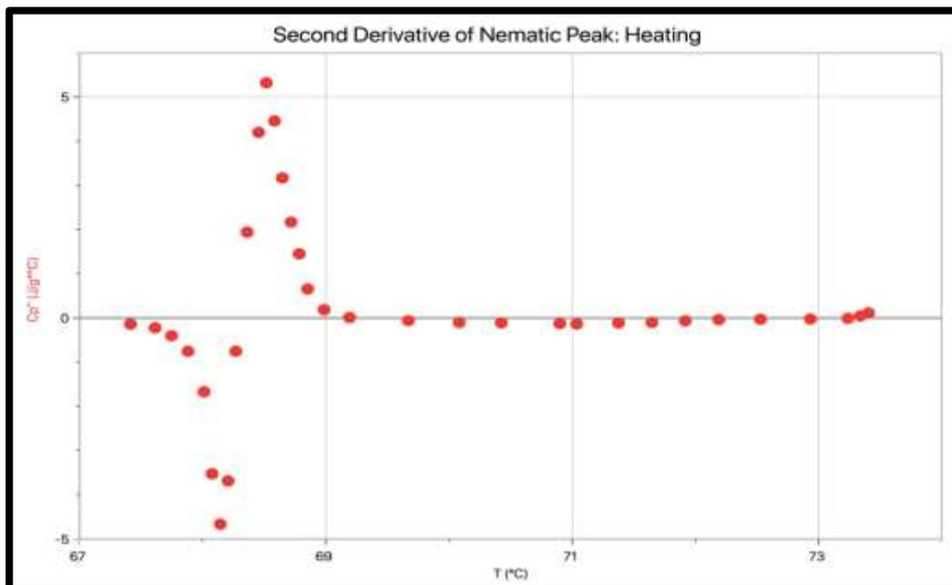
**Figure 15:** The second derivative of run 1's nematic peak during heating of 5OCB.
