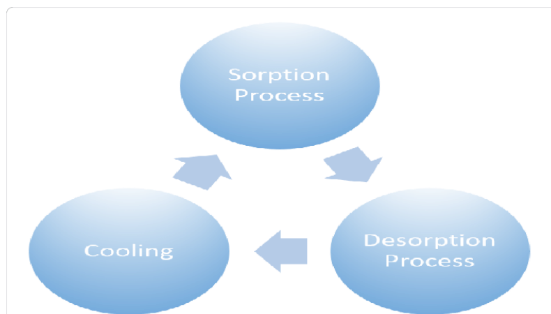
Figure4: Process of Moisture Transfer by Desiccant.
