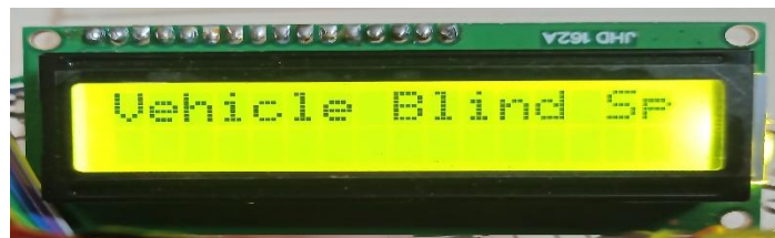
Figure 5: Blind spot warning on LCD
