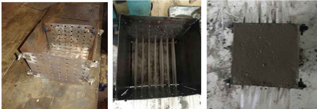
Fig 1. Mould showing fiber insertion Fig 2. Inside view of fiber concrete block Fig 3. Casting of block
