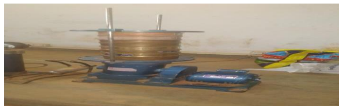
Fig4.1 : sieve analysis test
