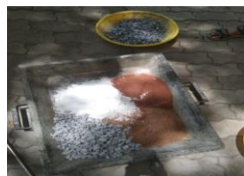
Dry mix of geopolymer concrete
