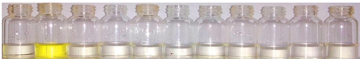
Fig.1 Visual changes of receptor ( 5.0 \times 10^{-5} M in 20:80 H 2 O: DMSO medium) upon adding 200 \mu L of anions ( 1.5 \times 10^{-3} M in DMSO)
