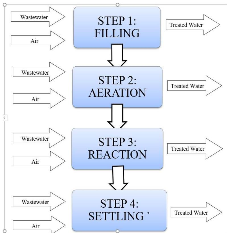
**Fig. 1** Flow chart of Moving Bed Sequential Batch Reactor
