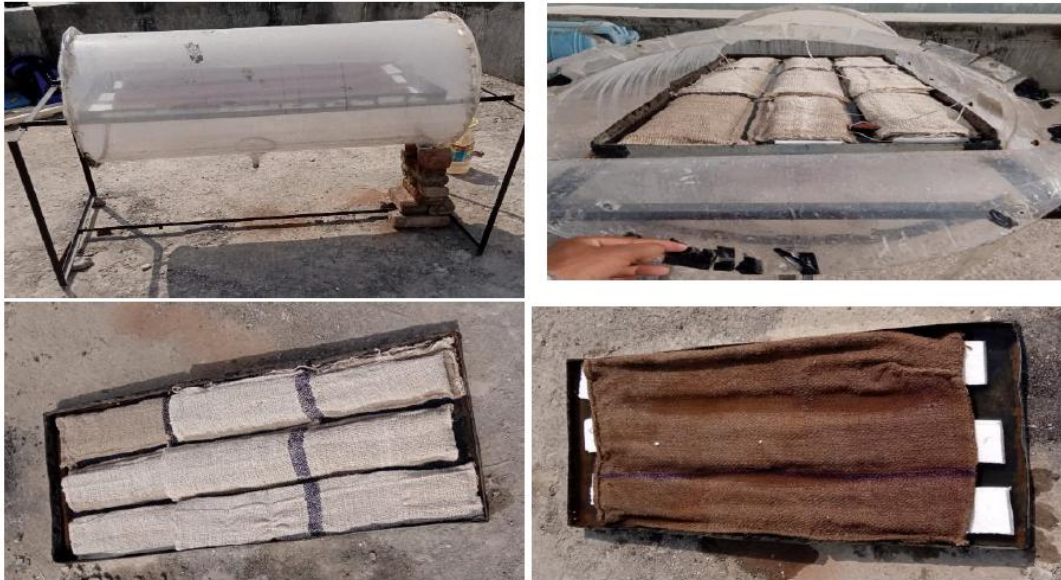
Fig.1 Experimental arrangements of TSS with wick materials (cotton and jute cloth)
