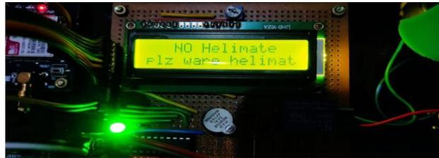
**Fig. 5: Message appears when helmet is not worn**
