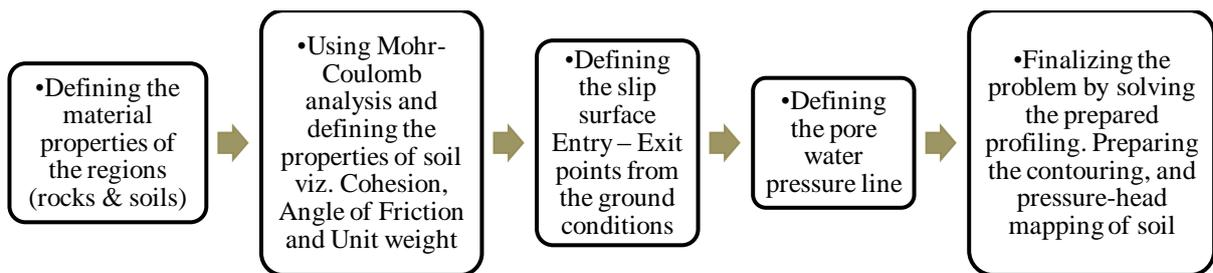
Figure 5 Completing the analysis and solving for the final results
