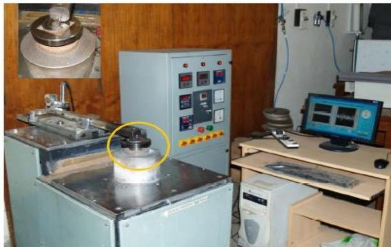
Figure 2 Photograph of pin-on-disc apparatus
