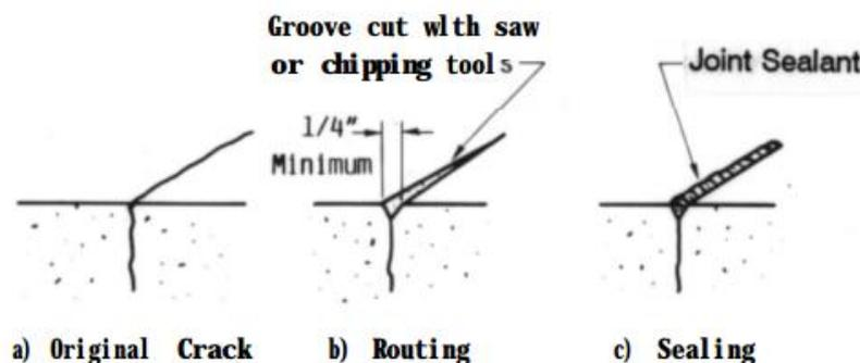
Routing and sealing is used to treat both fine pattern cracks and larger, isolated cracks. A common and effective use is for waterproofing by sealing cracks on the concrete surface where water stands, or where hydrostatic pressure is applied. This treatment reduces the ability of moisture to reach the reinforcing steel or pass through the concrete, causing surface stains or other problems.
