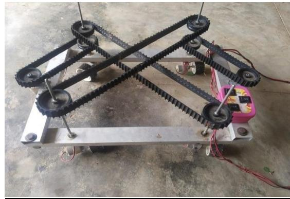
Figure show the fabrication of 90 degree wheel steering mechanism. In this project battery provides power supply to the control unit. The equipment contains six motors, two motors coupled with the vehicles left and two motors coupled with the right side of the front wheel, the next two are coupled to the vehicles left and right side of the back side.
