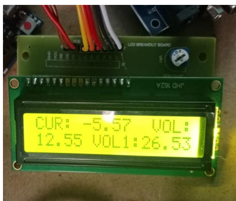
Figure 9: over voltage condition reading
