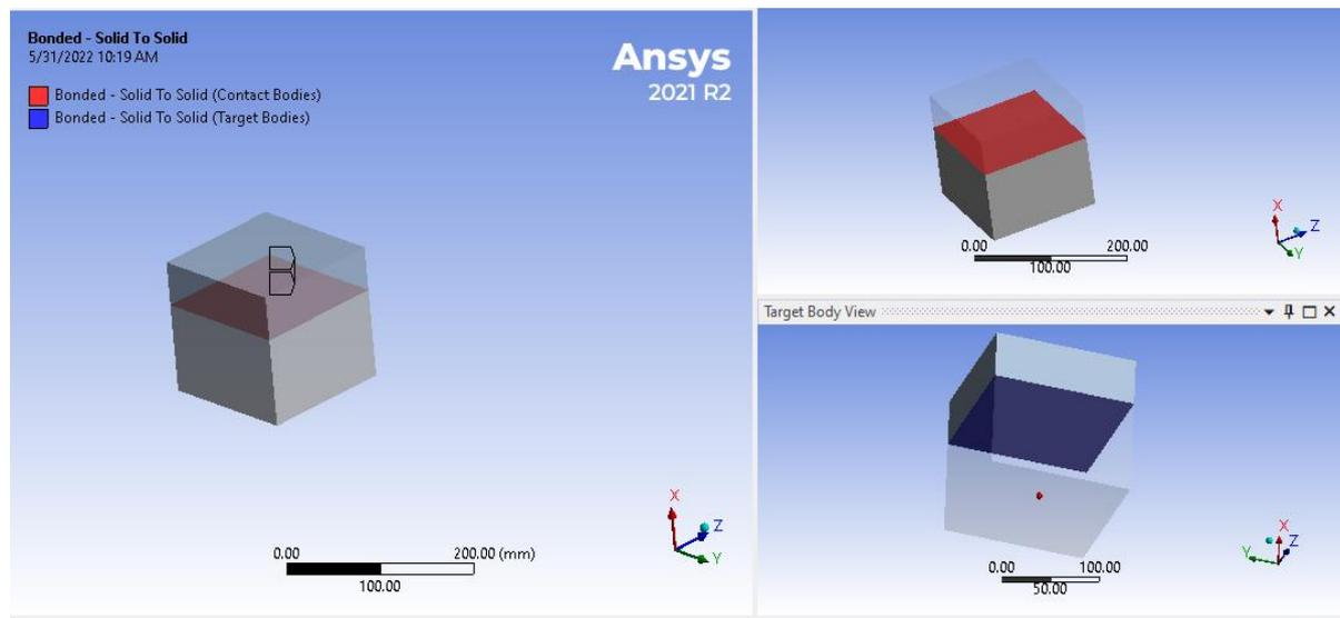
Figure 2: Model showing interfacial bond between FRC and UHPC with smooth surface conditions
