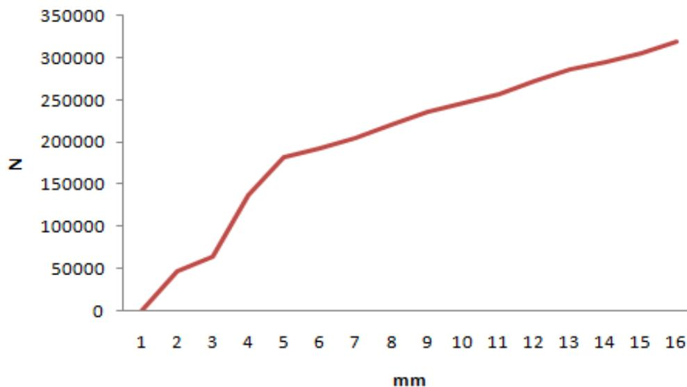
Figure 20: Displacement V/s force graph for rough surface connection between FRC and UHPC
