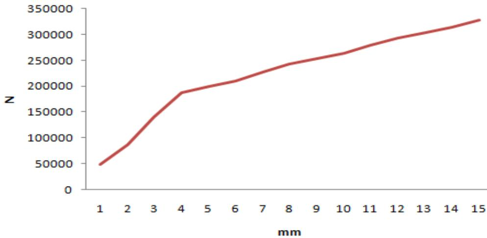
**Figure 10: Displacement V/s Force graph for smooth surface condition between FRC and UHPC**
