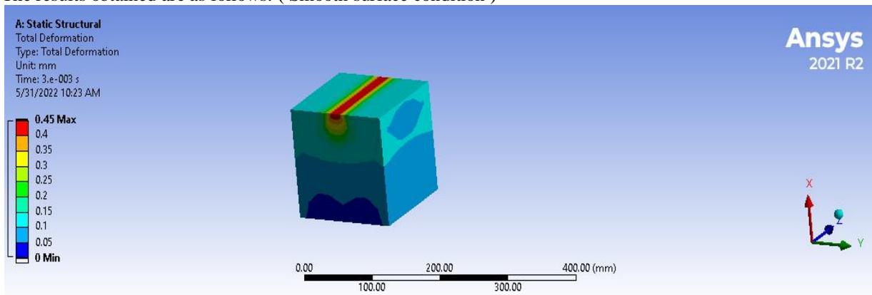
Figure 5: Total deformation pattern
