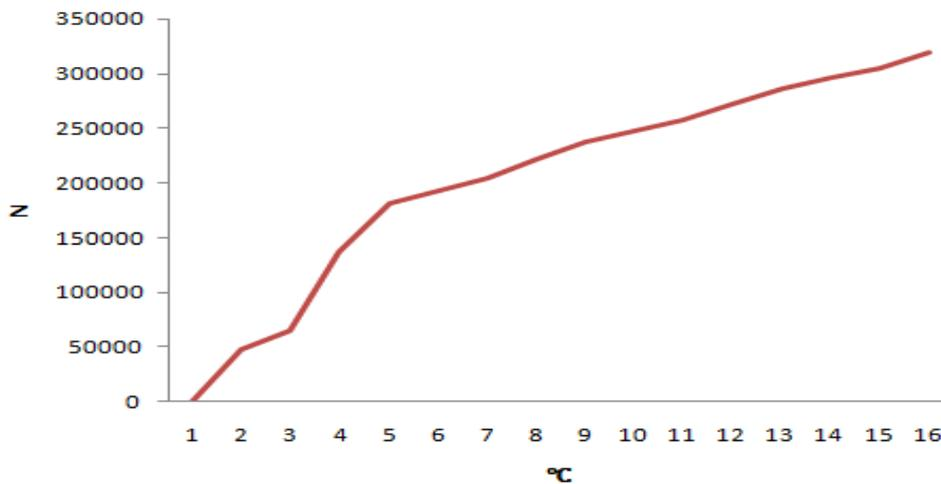
**Figure 21: Temperature V/s force graph for rough surface connection between FRC and UHPC**
