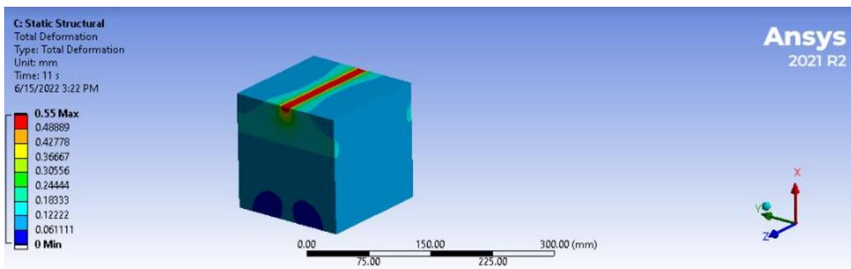
Figure 15: Total deformation pattern
