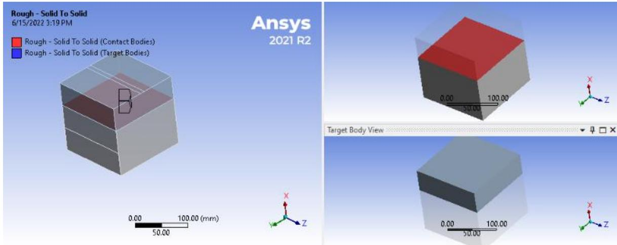
Figure 13: Model showing interfacial bond between FRC and UHPC with rough surface conditions
