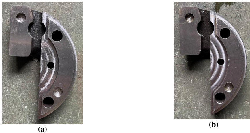
Figure 5. Machined surface of the tools for twisting and cutting steel rod \varnothing 6 with V=130 m/min, (a) f=90 mm/min, (b) f=60 mm/min
