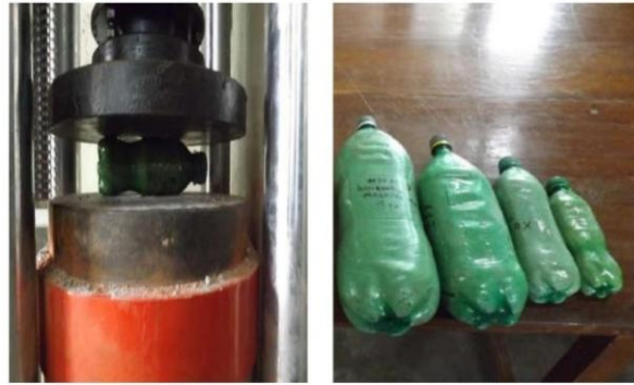
fig 6. Compression test for plastic bottle bricks and deformed bricks after the test
