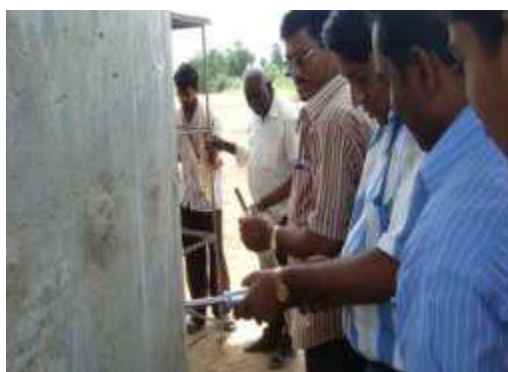
Figure 3: Testing of Bridge Pier using Rebound Hammer[1]
