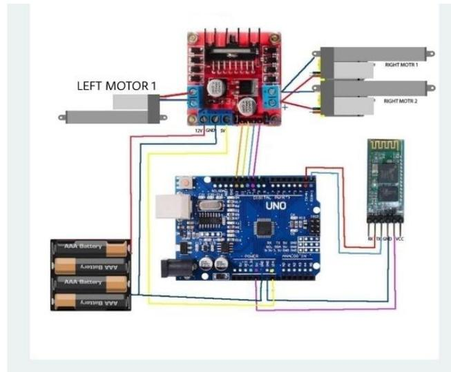
Fig 4.4: Wiring Diagram
