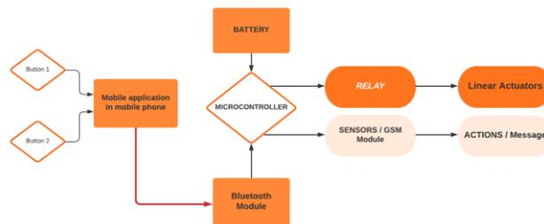
Fig 4.1: Block diagram of proposed automation
