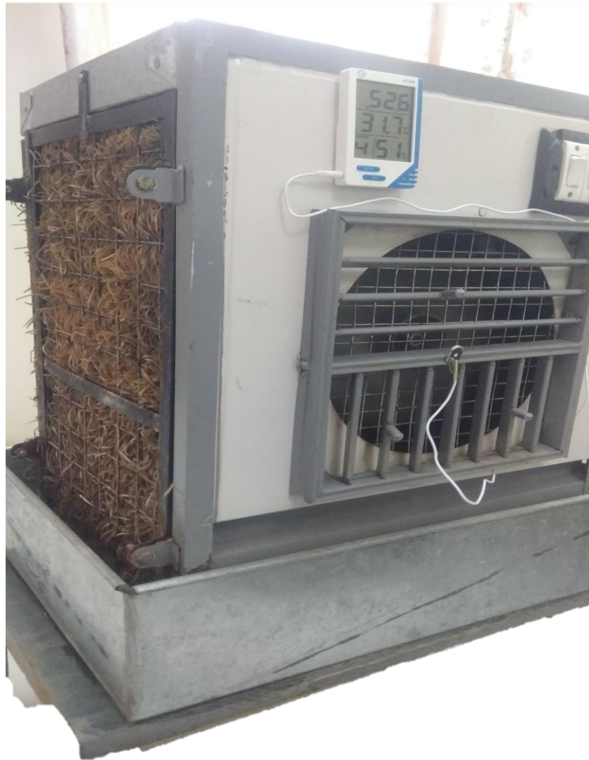
Fig.no.11 Experimental setup for wood wool pads. Temperature measurement using Hygrometer.
