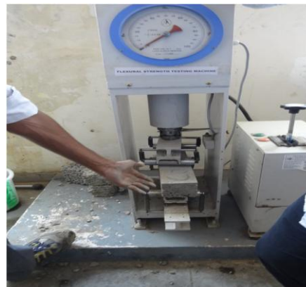
Fig :4 Flexural strength Test
