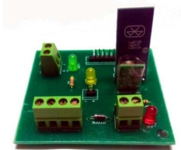
Fig. 6. PBC of controller of Underwater Robot (command transmitting part)
