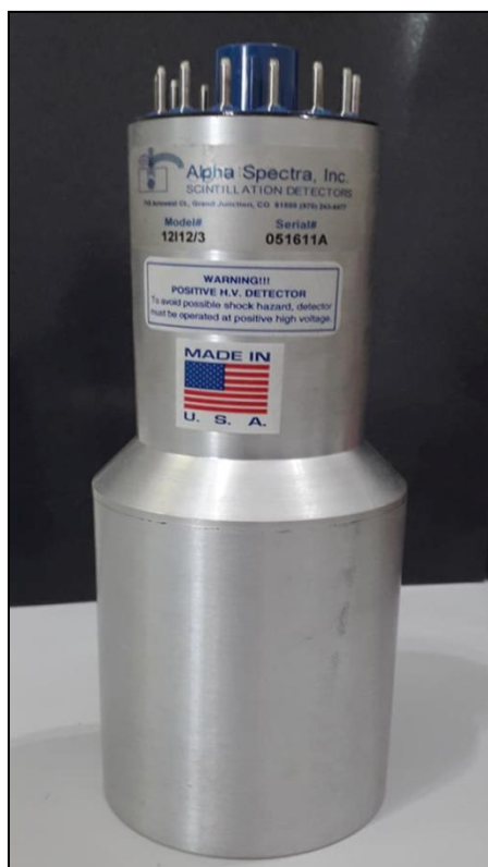
Fig. 5 - High precision Gamma Detector. Sodium Iodide crystal [NaI(Tl)]doped with Thallium.
