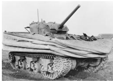
Sherman DD (Duplex Drive) amphibious tank with waterproof float screens. When in the water the float screen was raised and the rear propellers came into operation.
