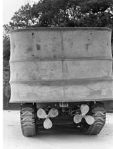
Rear view of a Sherman DD with its screen raised, showing the twin propellers in their lowered position
