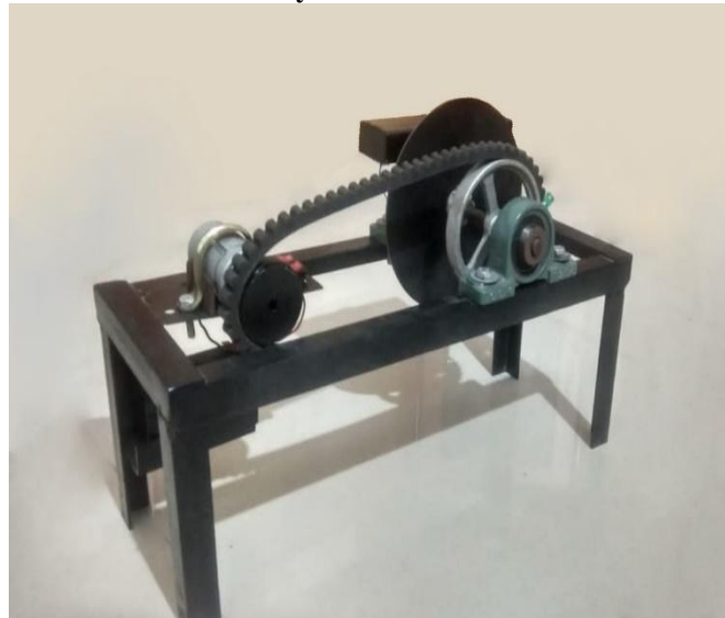
Fig 5.1 (Fabricated model of electromagnetic braking system)
